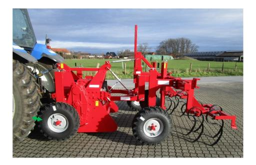
When mounting the rotary tiller at the rear, please note that the wheels of the tiller must be removed, as the distance to the tractor wheels is too smal.
