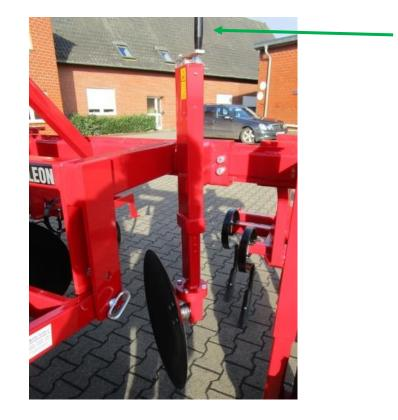
3. Setting the working depth on the rotary tiller
