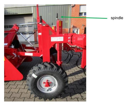
This setting also automatically controls the working depth of the tines.
