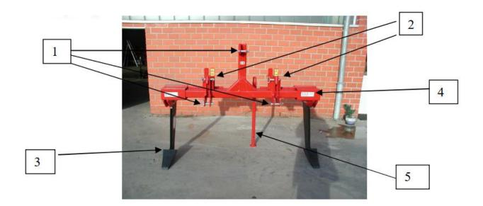
The depth spade MAULWURF has to be connected to the three point lever of the tractor (1).
